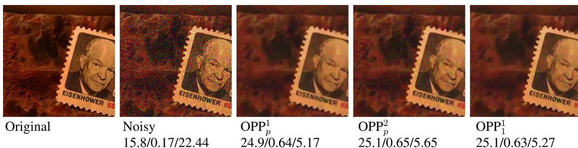
Fig. 9. Example result images from the evaluation dataset for standard deviation 60 of noise. OPP<sub>p</sub><sup>2</sup> performs well in images with piece-wise affine regions as indicated by the high SSIM value, although with respect to color consistency OPP<sub>1</sub><sup>1</sup> shows better result. (PSNR/SSIM/CIEDE).
