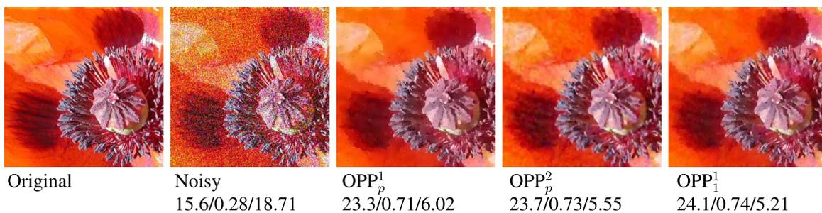
Fig. 8. Example result images from the evaluation dataset for standard deviation 60 of Gaussian noise. In this image the OPP<sub>1</sub><sup>1</sup> performs shows better performance than the non-convex counter-parts. (PSNR/SSIM/CIEDE).
