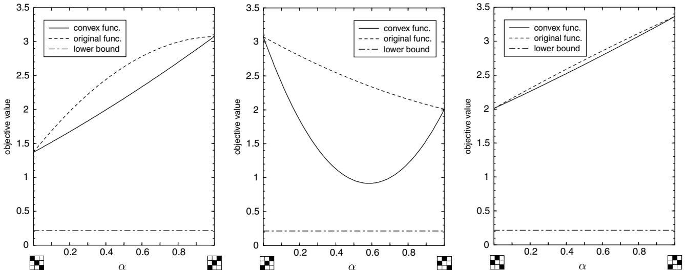
Fig. 3. The original objective function and its convex relaxation along paths through the relaxed solution set.
