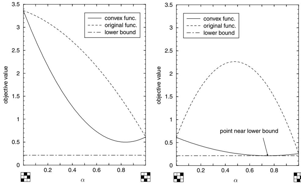
Fig. 4. The original objective function and its convex relaxation along paths through the relaxed solution set. On the right, the plot illustrates how the lower bound is attained at a point close to the global optimum (end-point on the right).
