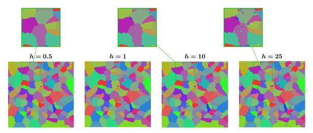
FIGURE 7.3. Visualization of regularization impacts when increasing the step size h corresponding to the results in Figure 7.2. Labeling results for various step sizes and the neighborhood size  $|\mathcal{N}| = 9 \times 9$ . Conforming to Figure 7.2, right panel, labeling accuracy quickly deteriorates once h exceeds the upper bound (5.3) (rightmost panel).
