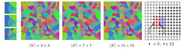
FIGURE 3.3. From left to right: Labeling results using (3.7) with the non-uniform parametrization (3.21), zero non-local Dirichlet boundary conditions and neighborhood sizes  $|\mathcal{N}| \in \{3 \times 3, 7 \times 7, 15 \times 15\}$ . Schematic illustration of the nonlocal interaction domain  $y \in \mathcal{V}^{\alpha}_{\mathcal{I}}$  (red area) induced by nodes (blue area) in  $\mathcal{N}(x)$  with  $|\mathcal{N}| = 5 \times 5$ . Using nonuniform weights (3.21) improves labeling accuracy.
