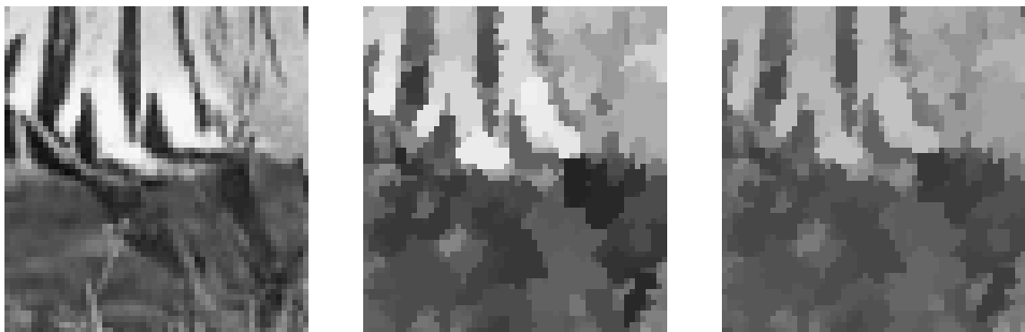
(b) Detailed view of the tiger denoising experiment revealing that contrast is better preserved when the Wasserstein term is used.
