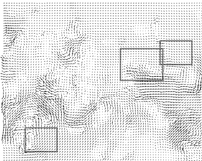
Fig. 14. Real 2D PIV experiment: Overview over the fluid flow, determined by our adaptive correlation method. A mean vector field of about 12 px to the right was subtracted everywhere. The rectangles mark the location of detailed views in – from left to right – Fig. 3, 16a and 16b.
