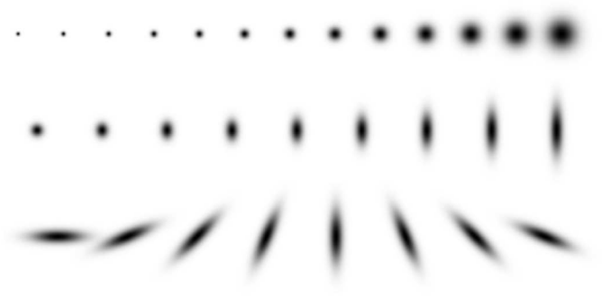
Fig. 5. Some possible shapes of the Gaussian weighting function as grey-value plot (white=0, black=1), from top to bottom row: varying radius, anisotropy and orientation
