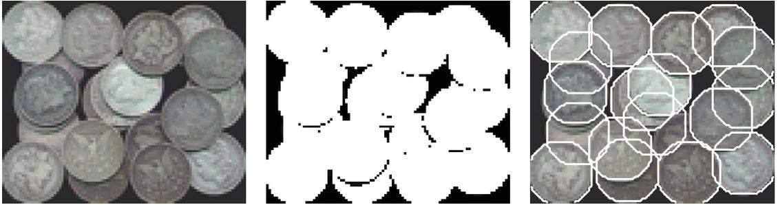
Figure 5: Application of the proposed approach to an image containing overlapping coins. Although not all objects are detected our approach reveals promising results and recognizes even highly occluded models. **Left:** Input image. **Center:** Local pre-segmentation obtained by inspecting the distance to the background color and local thresholding; used as input to the proposed method. **Right:** segmented result.
