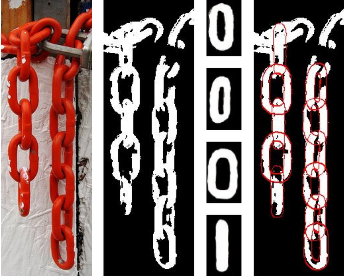
Figure 6: Application of the proposed template-based segmentation approach to a real world image. **Left to right:** Original Image, local pre-segmentation using a thresholded distance to the color red as foreground indicator, shape templates used for segmentation, and the final result. Note that even highly overlapping parts are labeled correctly.
