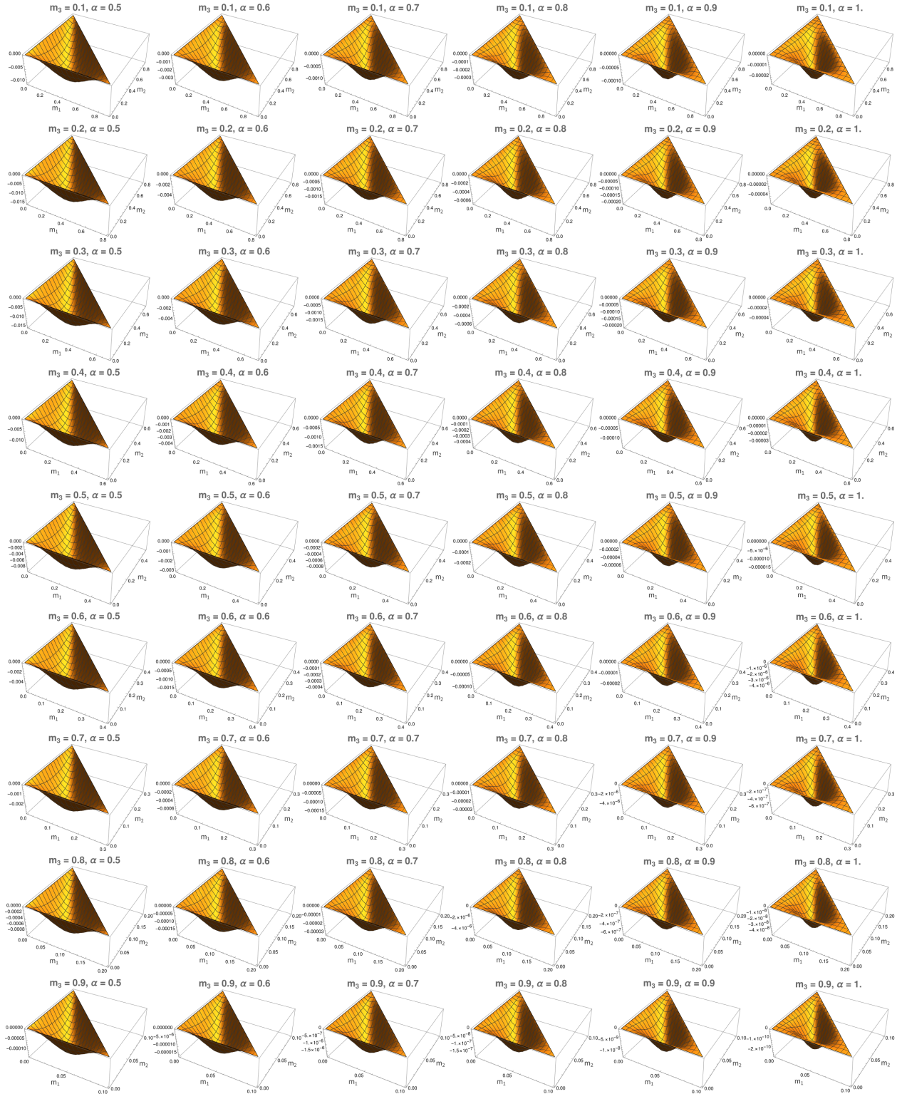
Figure 13: SPs of Degree-4 in the Plane are Likely not Feasible for \alpha \in ]0.5, 1[ . Surface plots are depicted, illustrating the left side of equation (16), as a function of m_1 and m_2 , with different fixed values of \alpha and m_3 . From left to right: m_3 is fixed and \alpha ranges over \{0.5, 0.6, 0.7, 0.8, 0.9, 1.0\} . From top to bottom: \alpha is fixed and m_3 ranges over \{0.1, 0.2, \dots, 0.8, 0.9\} . For m_3 fixed, m_1 and m_2 range over the domain defined by \{(x, y) : 0 < x + y + m_3 < 1\} . In all plots, the function values are negative and tend towards 0 as m_1 , m_2 , or m_3 approaches 0. We can observe that for fixed m_1 , m_2 and m_3 , the function seems to be increasing with respect to \alpha (from right to left). Since we have previously demonstrated that the left side of equation (16) does not equal zero in the desired domain for \alpha = 0.5 and \alpha = 1 , the plots suggest that this is also the case for \alpha \in ]0.5, 1[ .
